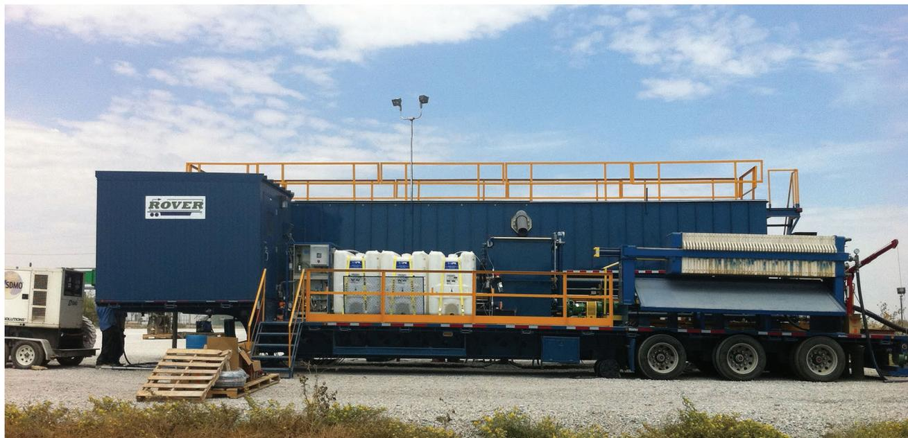
The ROVER mobile clarification system was developed for heavy oil applications and is used in treating hydraulic fracturing flowback fluids. Photo courtesy of Fountain Quail Water Management.
