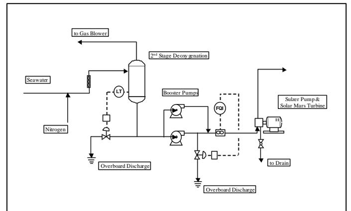
Fig. 6. WF2 Level / Flow Control System
