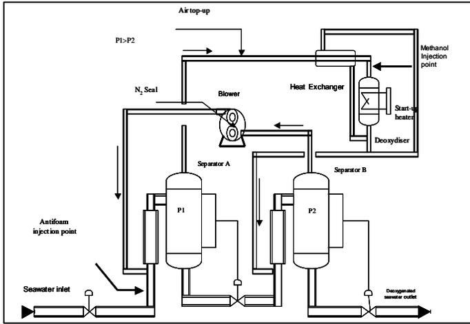
Fig. 1. Process Flow Diagram for the DeOx System
