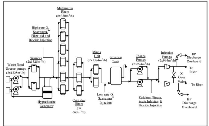
Fig. 4. WF3 Process Flow Diagram
