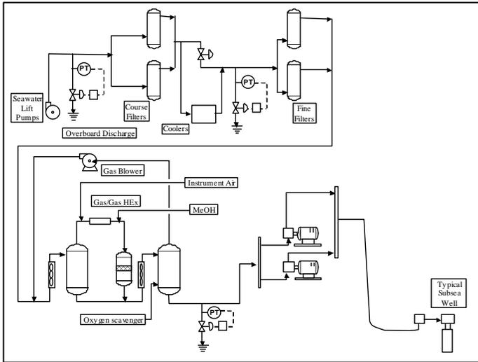
Fig. 2. WF1 Process Flow Diagram.
