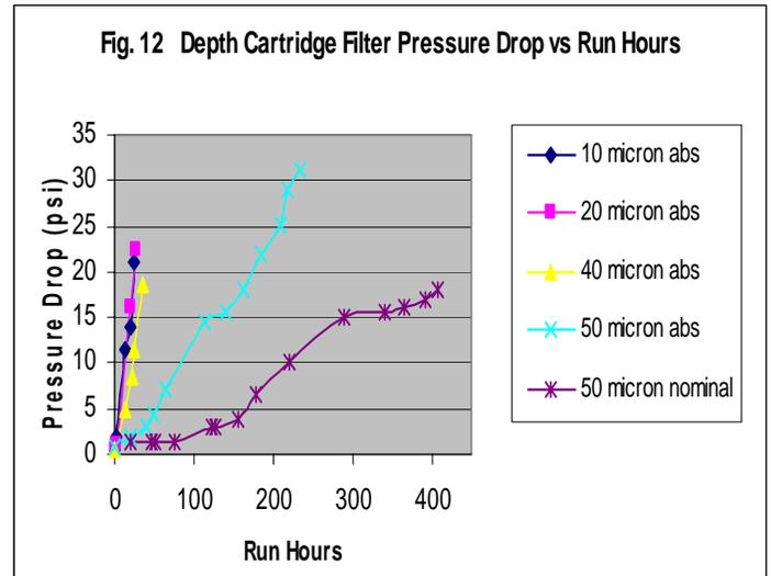
The pressure drop data for the two cartridge filters in series process was discussed earlier. The service life of the 10 micron absolute filter was increased to at least 500 hours if a 50 micron nominal filter was installed upstream to remove larger particles.
