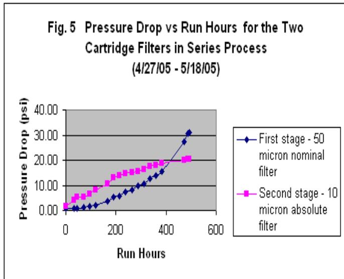
In this pilot project, both the filters were changed out when the first filter pressure drop reached 30 psi. For a commercial application, the second filter needs to be changed out only if its pressure drop rises to 30 psi.
