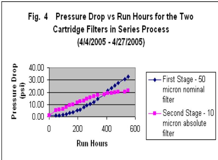
Once the pressure drops of the first stage filter reached greater than 30 psi, both the first and the second stage filters were changed out. The test was then repeated. The results of the next run from 4/27 to 5/18/2005 are shown in Fig. 5. The results of this run indicated that the pressure drop for both the filters are very similar to those for the previous results as shown in Fig. 4.
