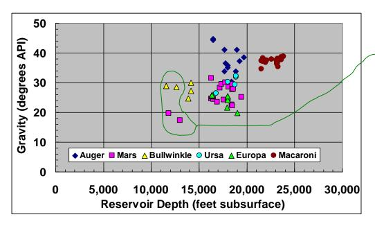
Biodegradation ceiling around 13,00 ft. Confirmed biodegradation for 2 Mars and 2 Bullwinkle wells - made water treating more difficult. Low API and high Total Acid Number (TAN) are indicative of biodegradation.
