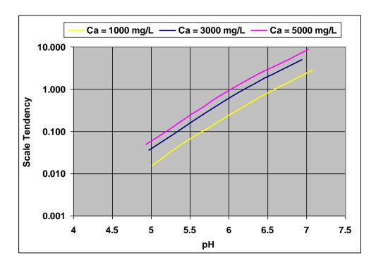
Calcium carbonate scale is common in E&P. Calcium comes from the formation water. Carbonate comes from dissolved CO2, and from bicarbonate in the formation water.
